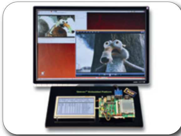
Figure 1. Complete Qseven system construction with display
