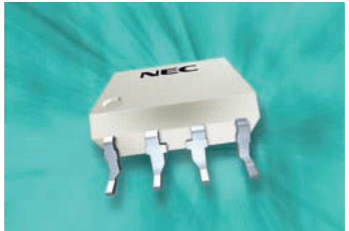
The optocoupler in its new white DIP package
